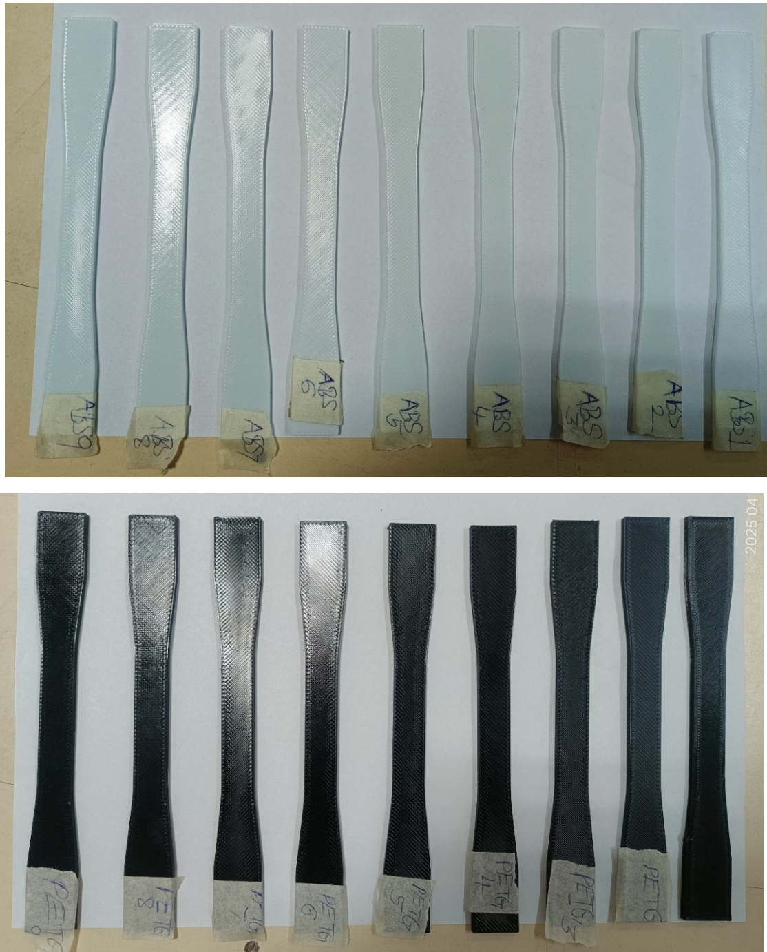
Fig. 2 3D Printed Tensile Test Specimens of ABS and PETg material based on ASTM D638
