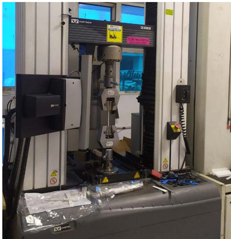
Figure 4. UTM for Tensile Testing at Narayan Industries & Technical Services Testing Laboratory, Kanpur
